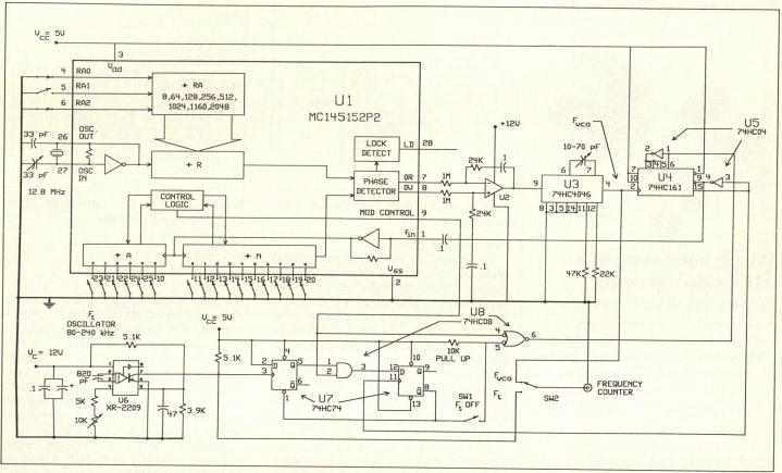
Figure 6. Proof of concept test set schematic.
