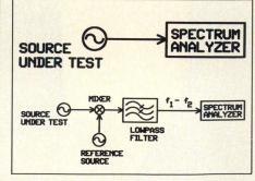
Figure 5. Two different phase shift measurement set-ups.
