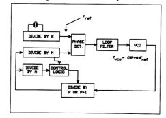
Figure 2. Dual modulus synthesizer.
