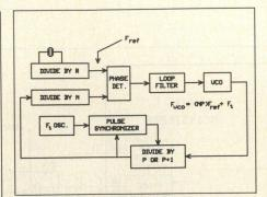
Figure 4. Infinite resolution synthesizer.
