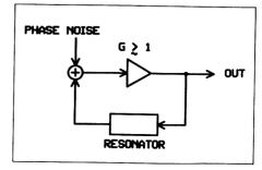
Figure 3. Phase noise injected into an idealized oscillator.
