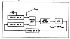
Figure 1. Single loop synthesizer with prescaler.
