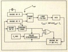
Figure 5. Infinite resolution dual modulus synthesizer.
