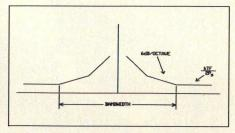
Figure 4. Predicted noise spectrum of an oscillator.
