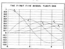
Figure 2. The first five integralorder Bessel functions. Note all functions vanish at zero except for the zeroth order.
