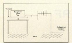
Figure 1. The basic setup for prequalification testing for radiated emissions. Tests use various antennas, test distances and equipment positions.
